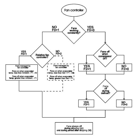
**N.B.** The broken lines of the diagram refer to the instruments with serial number greater than 100,000; see the following chapter "Notes for the new release" to a more detailed description of this parameter functionalities, effective for the instrument with serial number greater than 100,000).
