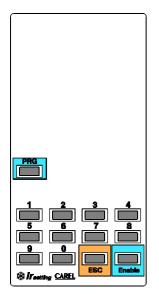
The buttons shown on the left are the remote control unit ON/OFF buttons. They also allow you to memorize any new parameter value.
