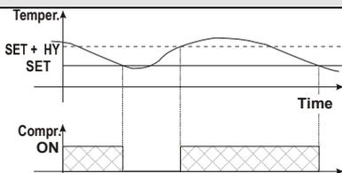
In case of fault in the thermostat probe the start and stop of the compressor are timed through parameters "CO<sub>n</sub>" and "CO<sub>F</sub>".
